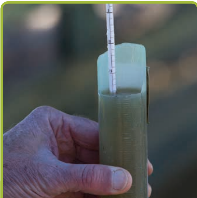
Hydrometer: A hydrometer measures the levels of chemicals in the dissolved solution and can be used to manage the zinc concentration levels in the footbath.
