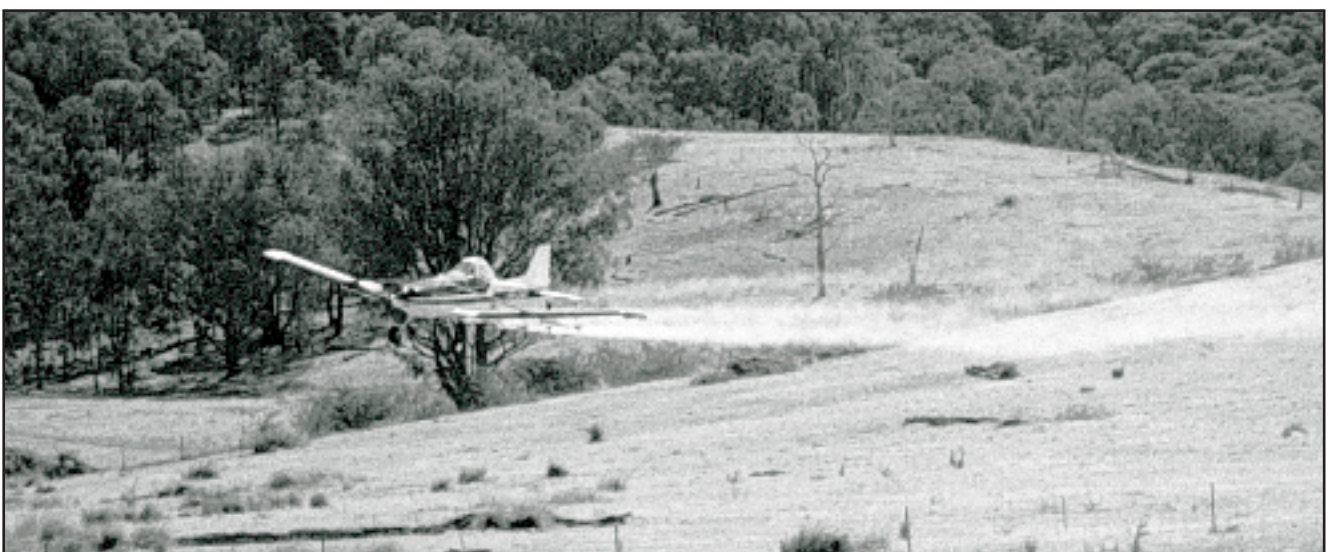
Aerially applying herbicide is the first step when using the aerial-spray-sow technique.
