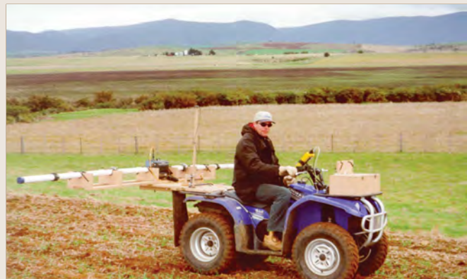
Plate 34 Quad bike mounted with combined EM31 and Global Positioning System (GPS) tracking system. Source: Department of Primary Industries, Parks, Water and Environment (2001)
