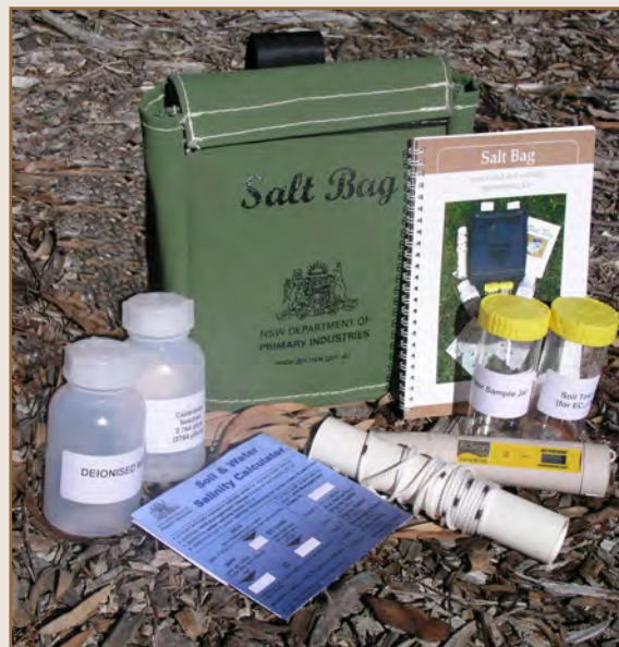
Plate 36 Contents of the Industry & Investment NSW Salt Bag used for salinity monitoring. Source: Madden, E. (2009)
