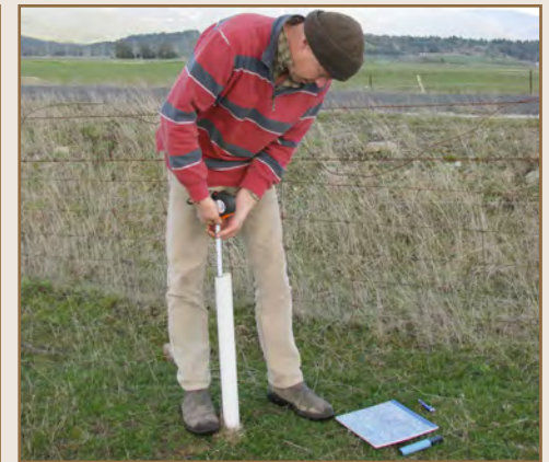
Plate 38 Measuring watertable depth using a monitoring bore. Source: Sherriff, L. (2009)
