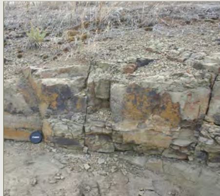
Plate 6 Fractured sediments (Triassic sandstone) displaying vertical and horizontal fractures, near Jericho. Source: Hocking, M. (2008)
