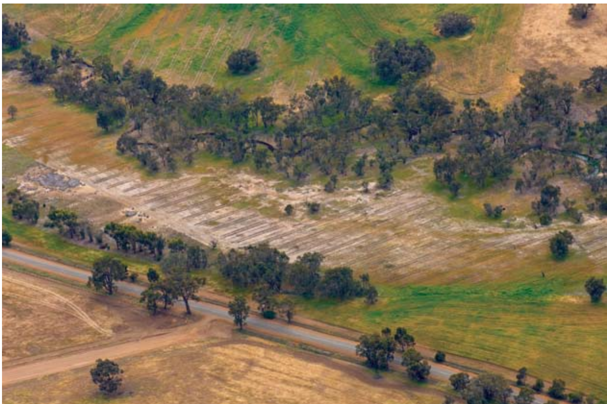
Aerial photo showing severity and variability in saltland.
