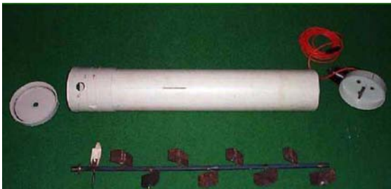
Figure 13. The Low Cost Seeder – showing internal working mechanism. [Photo: Keith Sanders].
