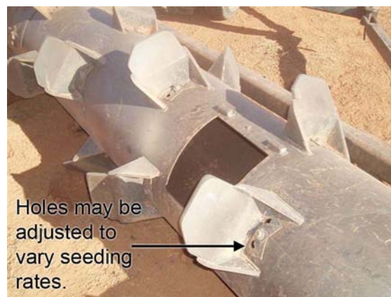
Figure 10. Crocodile drum seeder showing crude seed rate adjustment. [Photo: Paul Theakston]
