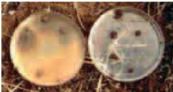
Placing soil into water can give a good guide to its stability. The soil on the left has dispersed when wet, while the sample on the right remains stable when wet.
