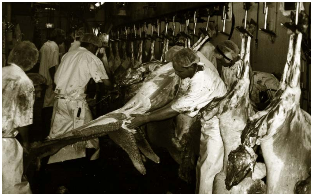
Processing mutton on an inverted slaughter chain
