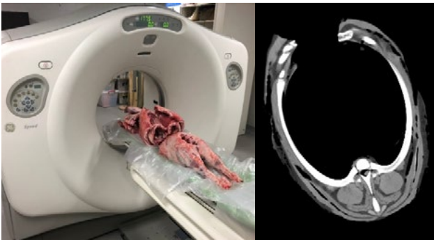
Figure 20. A lamb carcass being CT scanned to determine its lean meat yield and a cross-section CT image of a lamb fore section where the bone (white), meat (light grey) and fat (dark grey) can be clearly differentiated.
