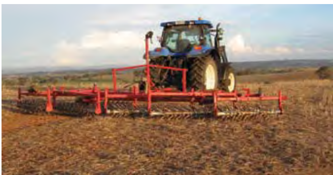
A rolling prickle harrow bar used to knock down stubbles and improve the decomposition potential for soil microbes.
