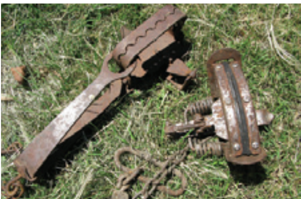
Pic. 31: Old style rabbit trap and new style with rubber padded jaws.
