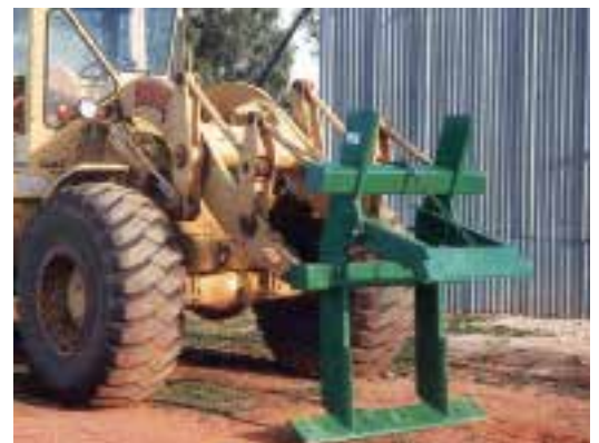
An example of a front-mounted grubbing unit
