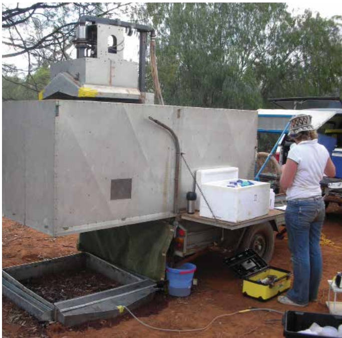
The erosion study's rainfall simulator in action.
