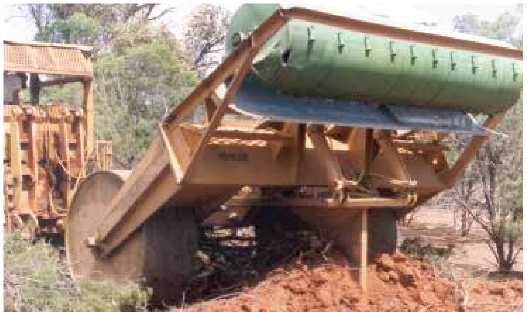
An example of a blade plough with a seeder attached
