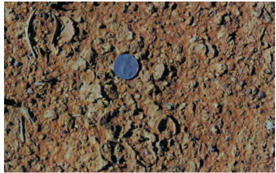
6a Soil surface extensively broken score 1, lower limit
