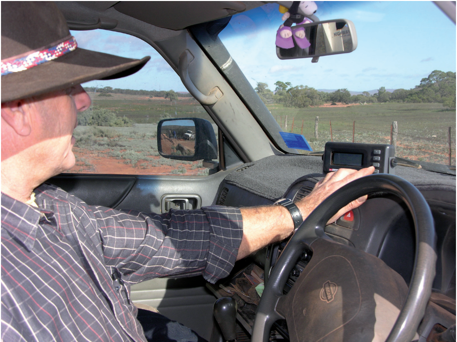
Figure 11: UHF unit in vehicle is used to remotely check water levels in tanks
