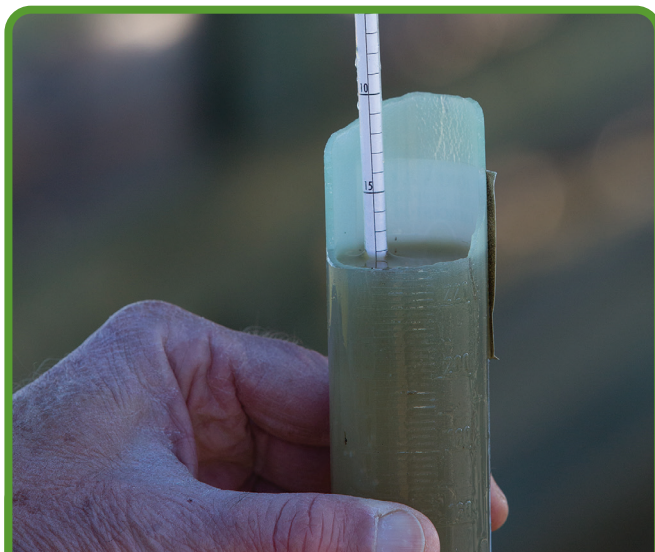
Hydrometer: A hydrometer measures the levels of chemicals in the dissolved solution and can be used to manage the zinc concentration levels in the footbath.
