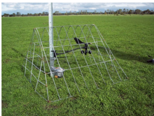
Figure 1. Wind speed meter set up in an unsheltered (control) paddock. The wind data was combined with Bureau of Meteorology temperature and rainfall data to calculate chill index.
